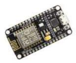
Fig: NodeMCU Development Board
