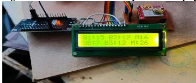
Figure 4 Output of the Bin levels, object detection values and moisture value of the objects
