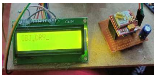
Figure 2 Dry waste detection output on lcd display
