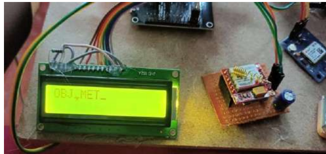
Figure 3 Metal waste detection output on lcd display
