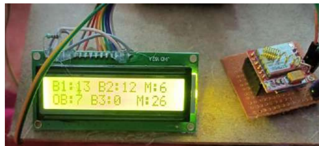
Figure 5 Output of the Bin levels , object detection values and moisture value of the objects
