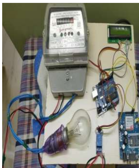
Fig.9 represents prepaid electricity energy meter before power su
