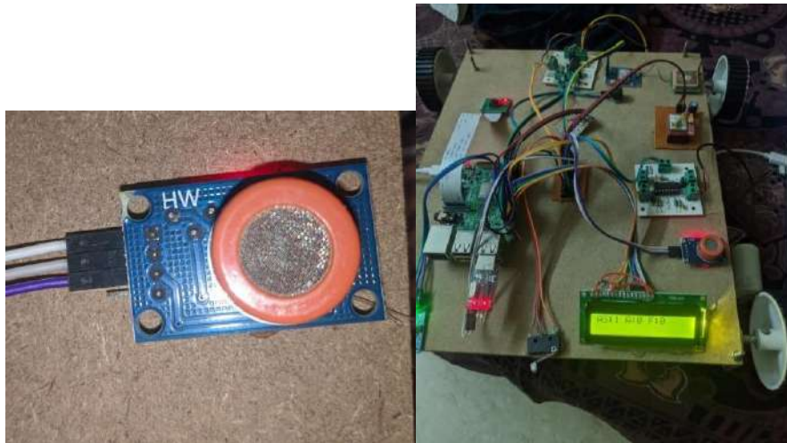
Figure 4: Detecting alcohol using the MQ3 sensor
