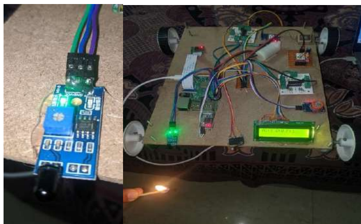
Figure 5: Detecting fire using the Flame sensor
