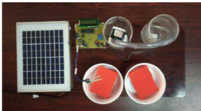
Figure.5. Hardware setup of the proposed irrigation system using solar power
