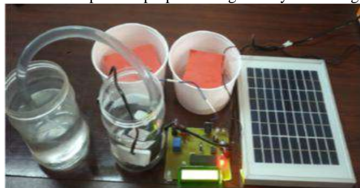
Figure.6. Operation of the Hardware setup of the proposed irrigation system using solar power under soil dry condition
