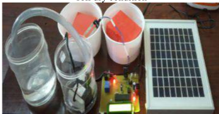
Figure.7. Operation of the Hardware setup showing soil dry condition and status of the pump in ON condition
