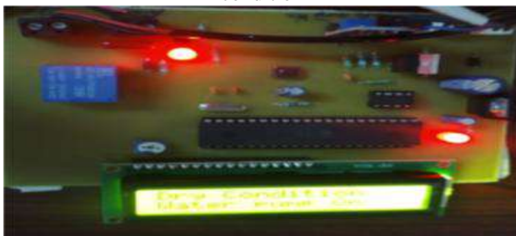
Figure.8. Operation of the Hardware setup of the proposed irrigation system using solar power under soil dry condition
