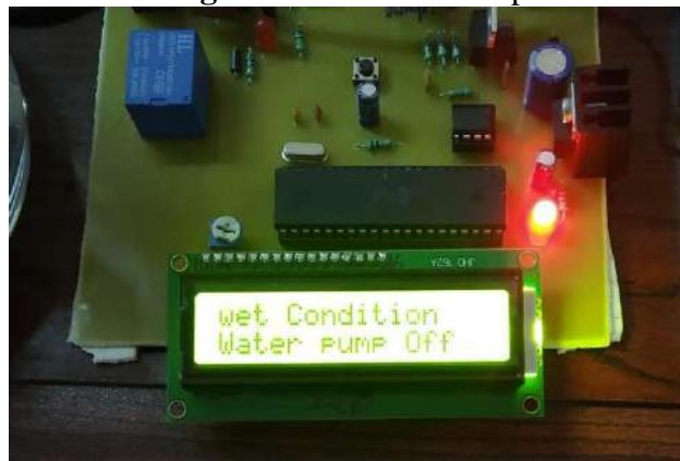
Figure 4 Operation of the Hardware setup showing soil wet condition and status of the pump in OFF condition
